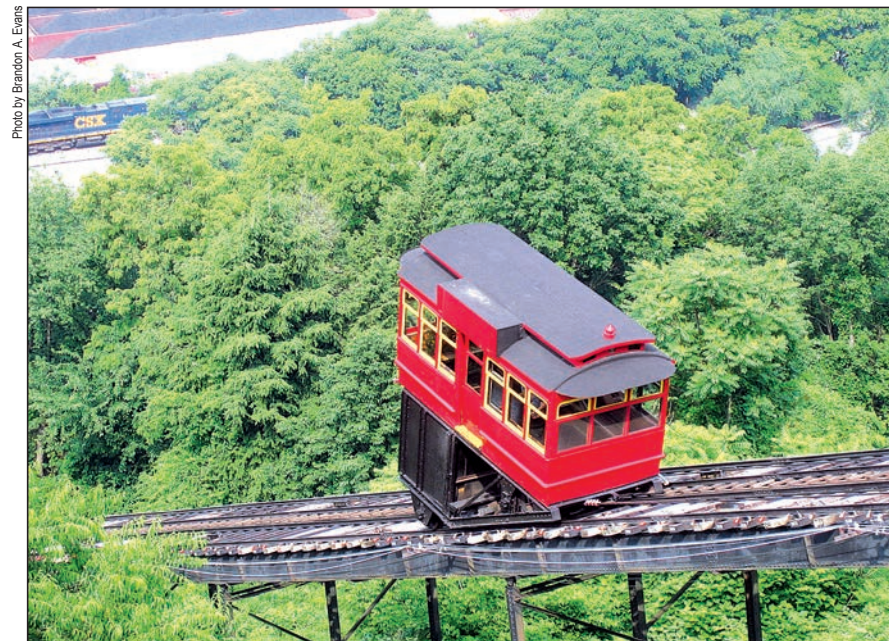
Above, the Duquesne Incline climbs the eastern face of Mount Washington in Pittsburgh. Opened for service in 1877, the Incline's track has a total rise of 400 feet on a grade of 30 degrees.
